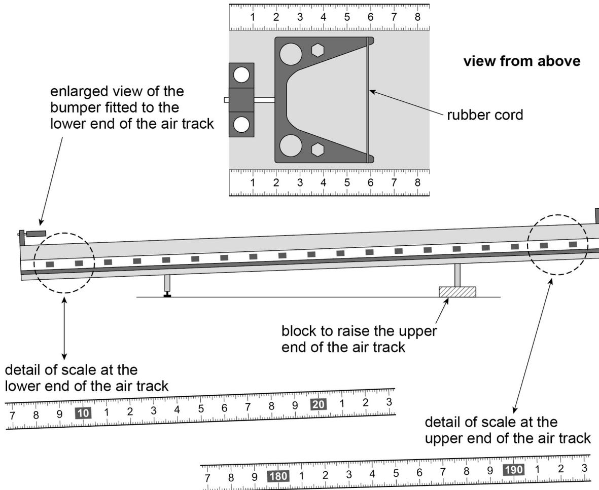
A glider is placed in contact with the rubber cord on the bumper at the lower end of the track. The position of the glider relative to the fixed scale can be determined using **Figure 14**.
