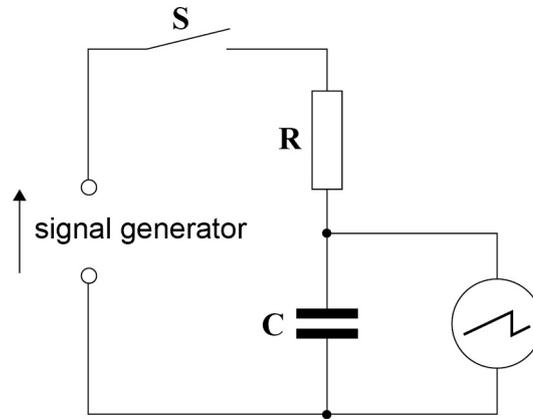
The oscilloscope is connected across the capacitor.
