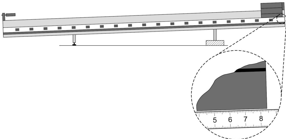
The air supply to the track is turned on and the glider is released. The glider accelerates down the track, strikes the rubber cord on the bumper and rebounds back up the track. The glider is allowed to bounce off the rubber band 20 times before it is stopped.
