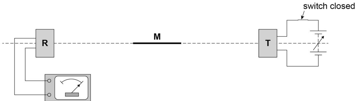
**M** is kept parallel to the marked line and moved slowly away as shown in **Figure 3**.
